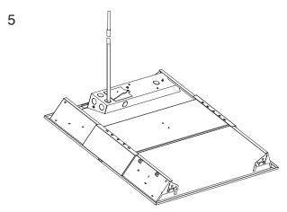
After the power cord is correctly connected, reinstall the access plate. Verify that the LED light works prior to installing into the ceiling.
