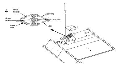
Connect the power cable wires to the wiring terminal through the opened knockout. Ensure that the wires have a strong connection.
