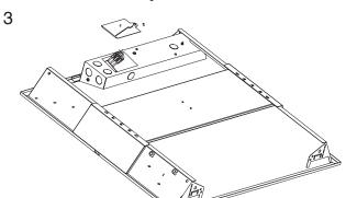
Remove the access plate. Open up one of the knockouts to allow the power cable into the driver box.
