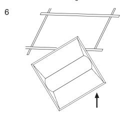
Install the fixture into the ceiling or designated space.
