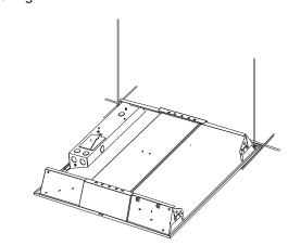
Attach the safety cables as necessary.
